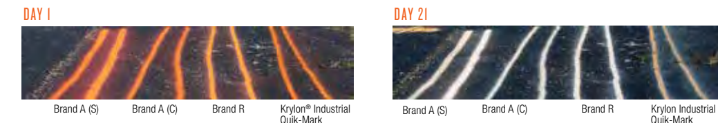
Per APWA color code guidelines, orange indicates phone lines, while white indicates proposed excavation
